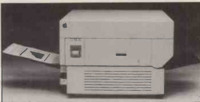
The Apple Laserwriter offers resolution of 300 dots per inch.
